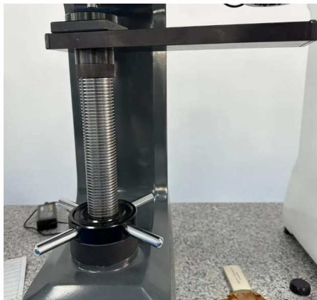
Slipped test table, frictionless screw
