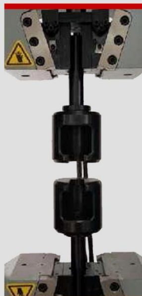
➤Grip for Fasteners (Bolt/Stud/Nut)
